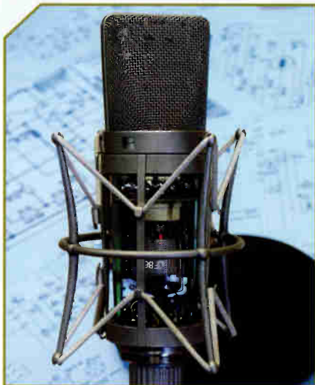
A Neumann U67 with EF86, a pentode wired as a triode
