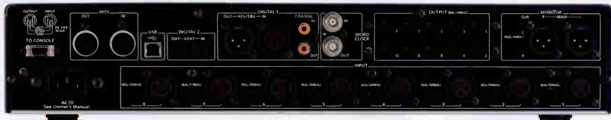
The V-700R provides I/O for the system, including phantom-powered mic preamps, digital I/O, word clock, MIDI and FireWire.
