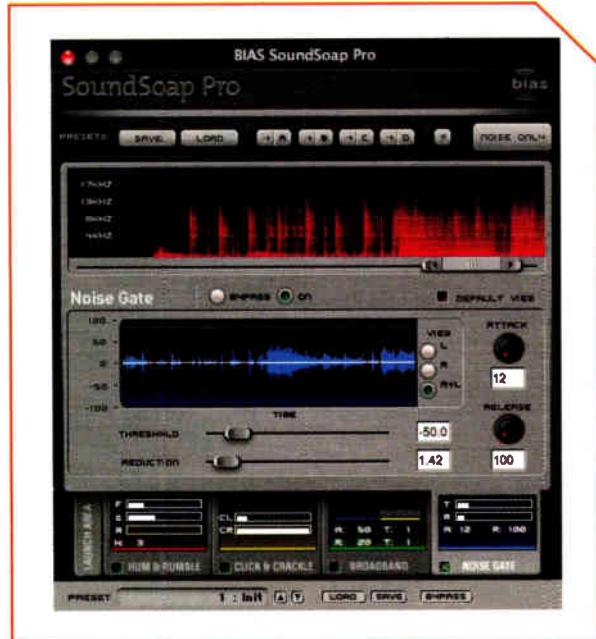
Figure 2: SoundSoap Pro combines hum, rumble, click, crackle and broadband noise-reduction tools.
