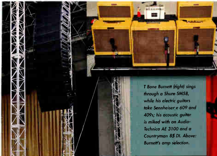
Roy Williams is pushing the co-headliners' lovin' sound through a Thunder Audio-supplied 24-box Meyer Sound system (above), which comprises 16 MICA side-hongs, HP-700s and M'elodie side-fills, and HP-700 subs; control is via Meyer Sound Galileo and SIM.
