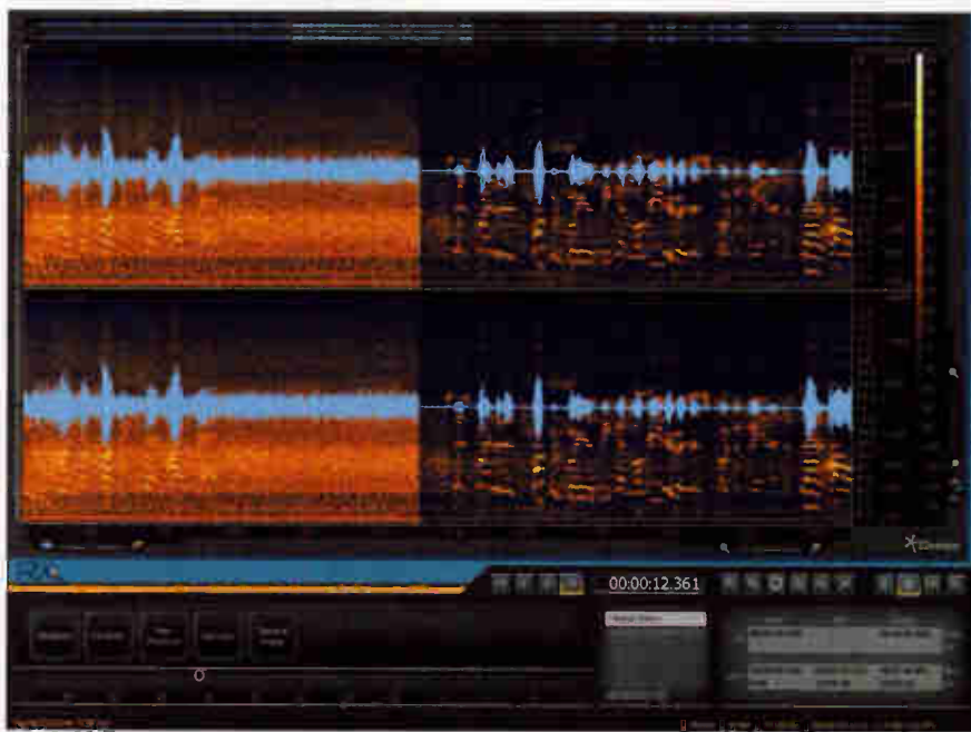
RX's main interface displays the currently selected region as a curtain of FFT spectral analysis with nearby zoom-view and waveform opacity sliders.
