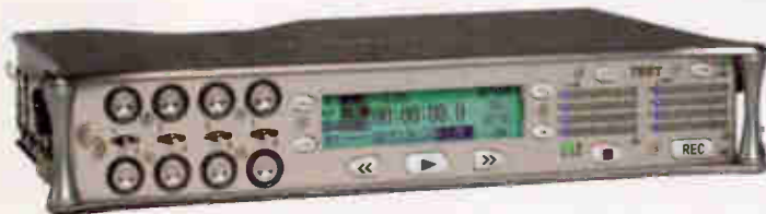
Sound Devices 788T location recorder can record to FireWire or USB.
