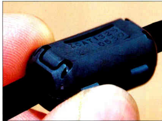
Figure 1: Ferrite clams go around the guitar cable just before the plug at the amplifier input.
