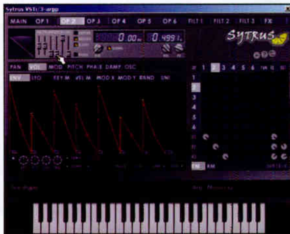
Sytrus' Algorithm/Route matrix (grid on right) routes operators.
