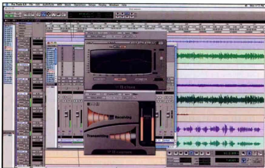
Using HTDMs in Pro Tools; up to 25 instances run comfortably on a dual 2.5 G5 or a P4 3.6.
