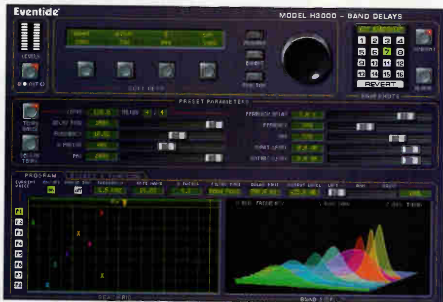
Band Delays offers eight tempo-based multi-tap delays, each with a programmable parametric filter.
