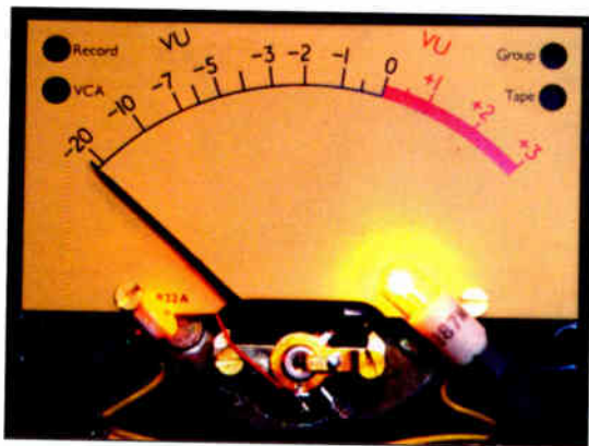
Figure 2: An SSL console meter with clear protective cover removed to access the lamps. At right, the incorrect Type 7387 bulb is installed (for comparison purposes); at left is an LED replacement.
