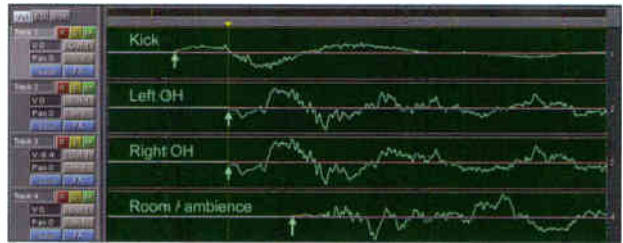
Figure 1: Time delay from kick, overheads and room mics
