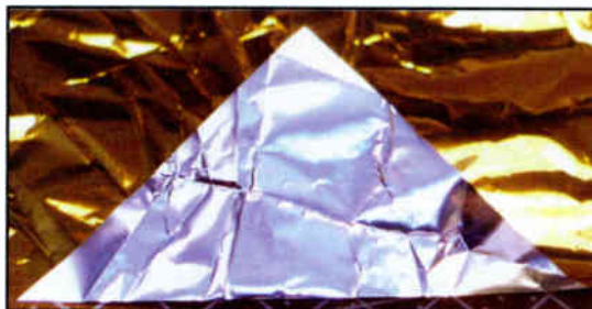
Fig. 2: a well-worn piece of space blanket material of the type used to replace the diaphragm on the CK-1 capsule. Note that the gold side is conductive, and the silver side is not.
