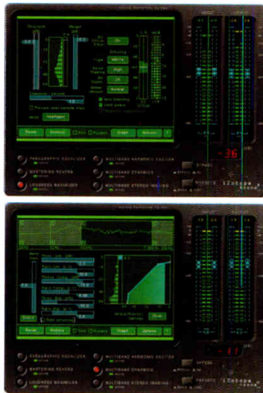
Ozone 3 processors include parametric EQ, multiband dynamics, multiband harmonic exciter, multiband stereo imaging, loudness maximizer and mastering reverb.
