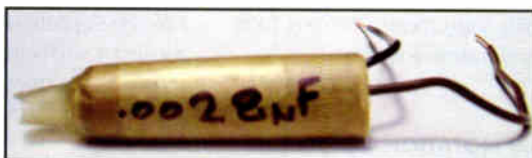
Fig. 1b: the assembled and tested capacitor
