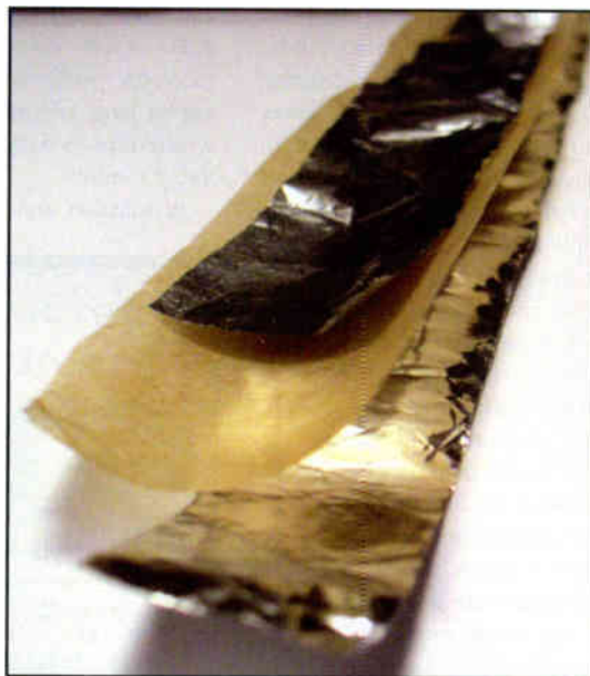
Fig. 1a: (above) raw materials for D.I.Y. capacitor
