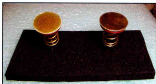
Fig. 3: on the left, an AKG CK-1 capsule "exposed," and on the right, the D.I.Y. diaphragm using a piece of space blanket material that is available at your local science museum's gift shop. The diaphragm connects to ground via the case, and the backplate connects to the amplifier, which supplies a polarizing voltage via the gold-plated spring and contact point.
