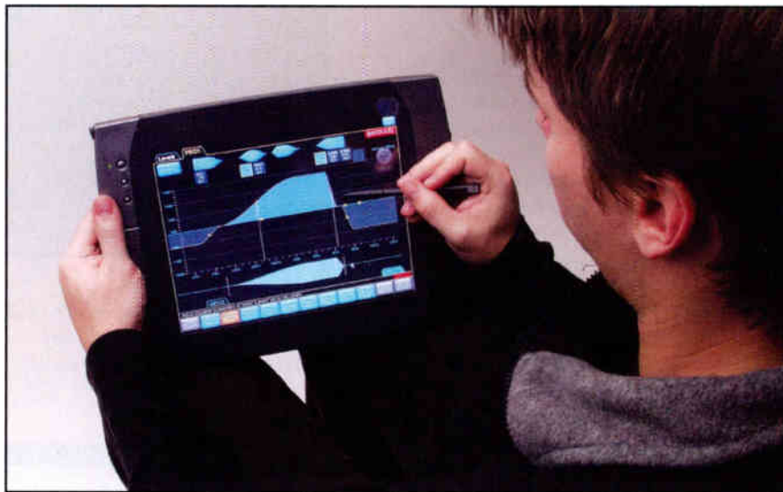
Lake Contour includes a WiFi touch screen tablet controller with many useful drag-and-drop functions.
