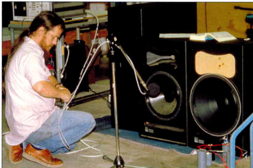
John Meyer, circa 1985, running FFT analysis of 500 Series prototype.
