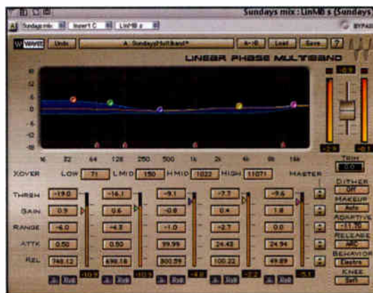
Linear Phase Multiband's Auto Makeup function should always be applied before using its Trim function. Never click on the Trim readout before a mix has played all the way through to its end, or while working offline.
