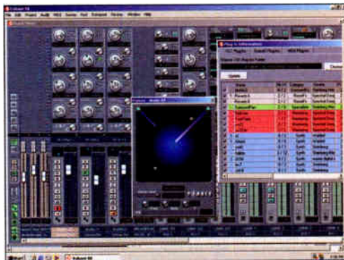
Figure 3: The surround panner can replace the mixer channels' stereo panners when the user is working in a surround project.
