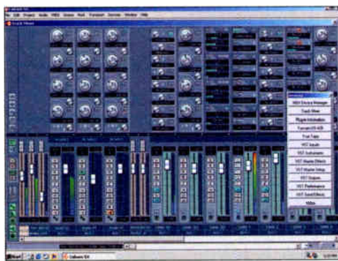
Figure 2: Mixer channels can be arranged in a variety of configurations, including narrow, wide and having different control configurations above a fader.
