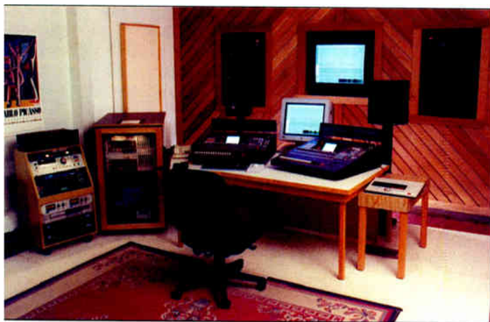
Studio A features two Yamaha O2R consoles and a Pro Tools |24 MIXplus system.
