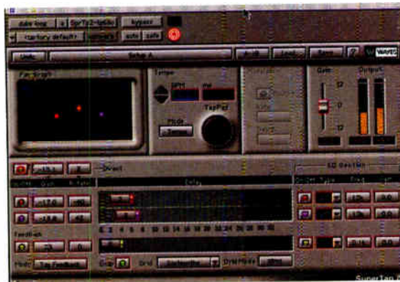
SuperTap comes in 2-tap and 6-tap versions, each with its own gain, panning (or rotation), EQ and delay.
