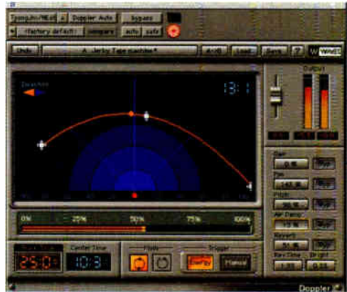
Doppler lets you adjust the effect's fly-by time, plus adjust reverb, panning, pitch shift and air-damping parameters.
