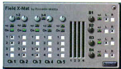
XMAT setup for the I configuration with a cardioid, a shotgun and a bidirectional mic. Bus 3 is phase-reversed.
