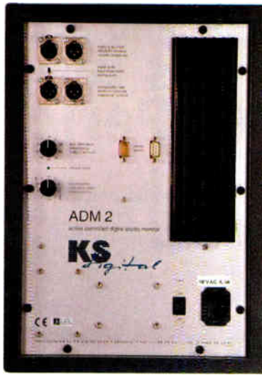
The rear panel features XLR I/Os and a toggle that switches between analog and digital audio in.
