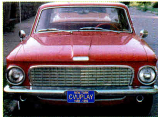
Figure 1: The stock 1963 Plymouth Valiant was equipped with a 220-cubic-inch slant-six engine, push-button automatic transmission and an AM radio with Class-A output amplifier. Fuel consumption was at least 20 mpg highway.
