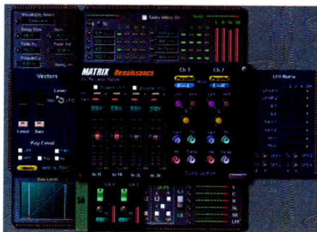
The Matrix. The Filter Mode buttons under the "Ch 1" and "Ch 2" legends in the main center section allow the HPF and LPF filters to be applied in flexible and unusual ways, while the parameters can be modulated by the LFO Matrix to their right.
