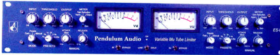
The ES-8 Variable Mu Tube Limiter employs six ES8 tubes, one per channel.
