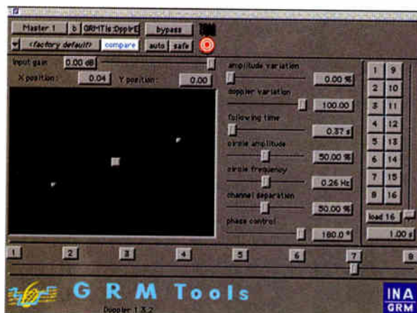
The Doppler plug-in lets you control passing speed, amplitude change and pitch change.
