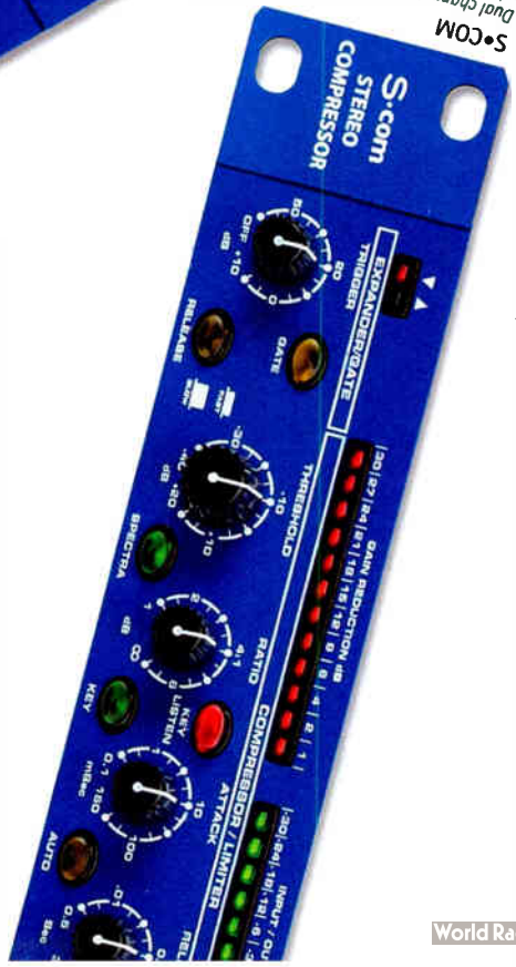
S•COM PLUS Stereo dynamic processor featuring dynamic processor, expanding gate and de-esser.
