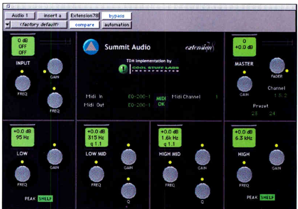
The Extension 78 TDM plug-in controls the MPE-200 and MPE-200S preamps via MIDI; it can be used with any sequencer that will run Digidesign's DAE engine, such as Emagic Logic Audio and MOTU's Digital Performer.
