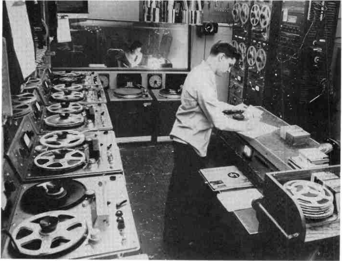
These Ampex machines are used to play tapes for programs over the FM stations and the city-wide wire network. Turntables are for taping discs
