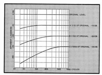
Fig. 2. Fall-off in apparent loudness of frequencies below 1,000 cycles as the volume at 1,000 cycles is cut down 10, 20, and 30 db below the level of the original sound
