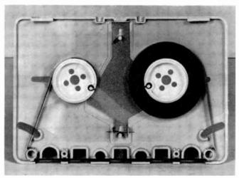
The RCA cartridge holds up to one hour of music on two-way stereo tape, running at 3¾ ips. Plastic case measures 7 by 5 ins., and is ½ in. thick.
