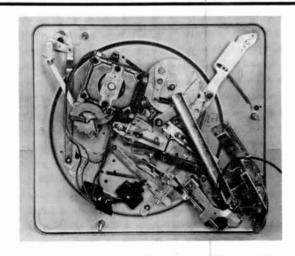
The record-changing cycle is the same at all turntable speeds, as the mechanism is driven directly from the motor. A muting circuit is put across the pickup during the change cycle.
