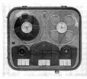
Award No. 58: Norelco 3-speed tape recorder, made in Holland. Most of the mechanism shown here of the top, rear, and sides is employed for pushbutton controls and interlocks. The three buttons at the left are for playback with a safety button above, and pause. The last, used for editing, stops the tape but
