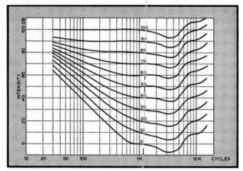
Fig. 1. Intensity levels required at various frequencies to equal loudness values of 0 to 100 db at 1,000 cycles. Zero db is a barely audible sound
