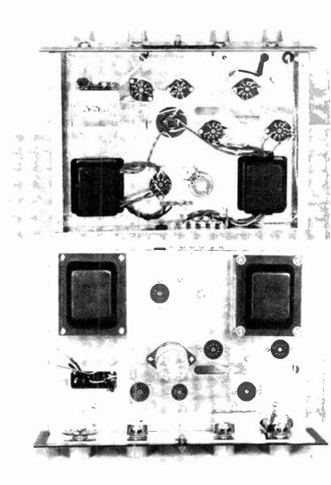
Left: Here the wiving is complete, as shown in pictorial diagram, No. 3. This stage is mostly a matter of adding capacitors and resistors, and soldering their leads to terminals, previously fastened to the chassis.
