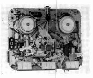
not the motor. At the center are controls for rewind, stop, and fast forward. Speeds of 1%, 3%, and 7½ ips. are selected by the buttons at the right. There is a mike jack on the top of the chassis, and jacks at the side for an external speaker, radio or phone input, and a high-impedance output for a hi-fi system. Price with microphone \$269.50
