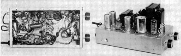
Award No. 61: Dactron Steradapter for 2-track stereo tapes. Designed to convert any monaural tape machine to stereo playback operation, this unit is so simple and inexpensive as to make one wonder if it can be really good. After a year of checking one of the Steradapters in regular use, we can report enthusiastically on its excellent performance.
