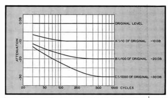
Fig. 3. Action of a typical loudness control. As the volume at 1,000 cycles is cut below the level of the original sound, there is less attenuation of the lower frequencies
