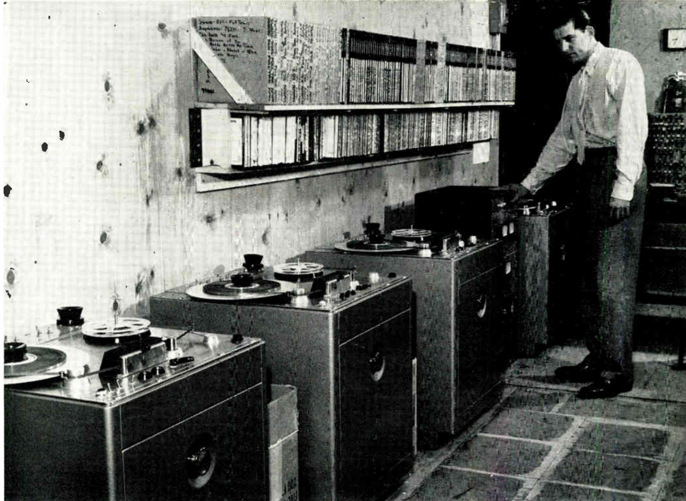
Output of the playback machine is fed to slave recorders. All machines run at 60 ips. Operator can spot-check quality of any tape copy
