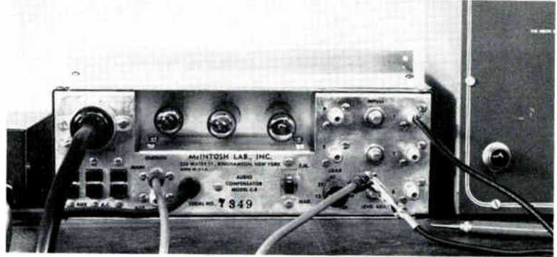
Fig. 2. Rear view of the preamp, with the output of the oscillator plugged in at one of the input jacks, and a lead brought from the preamp output for connecting the clip and prod of the meter. It is important to study the preamp instructions carefully, so that the connections will be made in the right way. Otherwise, the tests may be misleading
