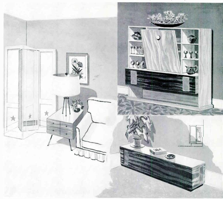
the top. The appearance is improved by using a base frame set in  $1\frac{1}{2}$  ins. This construction, fitted with a long cushion, can be used as a window seat. The end vent, about the size of the Air-Coupler port, is necessary because the space behind the speaker should not be sealed tightly.
