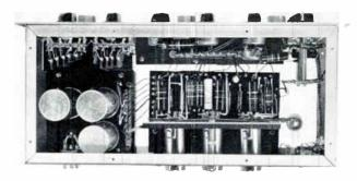
was photographed upside-down. On the top are three receptacles for plugging in other equipment, all of which can be turned on and off from switch\_on the front panel of the preamplifier, via the power cable
