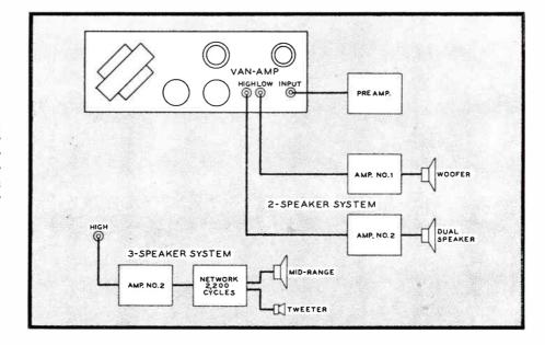
Fig. 9. With two speakers, each is driven from its own amplifier. With three, the high-range channel must he connected to a fixed network which feeds the mid-range speaker and the tweeter
