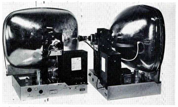
Fig. 6. Picture-tube chassis for remote-control operation. Pin jack at the left runs through the cable to cathode follower on the remote unit
