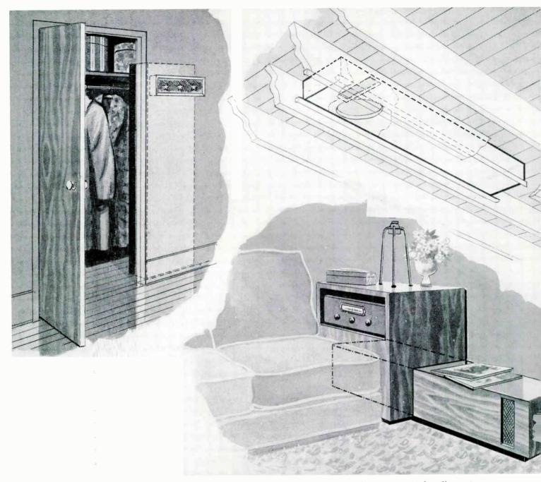
Fig. 8. If there is a closet in the room, it is an ideal place to mount the enclosure. Only construction required is an opening in the wall, opposite the port. Fig. 9. This is a very practical corner arrangement. Fig. 10. Beams under the living-room floor offer a most convenient mounting
