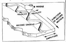
This diagram helps explain why, using Sonotone ceramics, you get a flat response without an equalizer. With a velocity type pickup, the voltage output will be 30 times as great at 10,000 cycles as at 50 cycles. It responds to side-to-side speed of needle movement. But our ceramics work on the "amplitude" principle-they respond to the amount of side-to-side movement.
