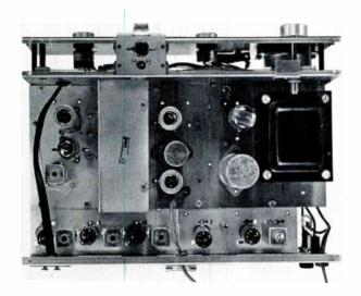
Inside views of the H. H. Scott FM tuner. In this pancake design, the tubes are mounted under the chassis, so that the photo above is actually the bottom view. For extra noise suppression, this tuner has three limiter stages. Note the instructions and tube layout printed permanently on the rear of the chassis
