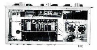
These views of the Marantz preamp show unusual attention to construction detail, precision workmanship, and ease of access to all the components. The separate unit containing the power transformer and rectifier
