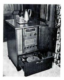
Fig. 1. A very simple appearance is achieved with this custom-built cabinet, by the elimination of all controls. Note that the picture tube is at a comfortable viewing height
