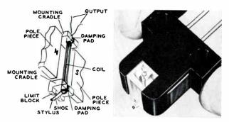
In the Electro-Sonic pickup, current is generated as the lateral movement of the stylus rotates a coil mounted in a magnetic field
