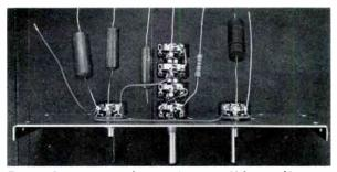
Fig. 6. Connections to the potentiometers, fifth assembly stage, must be made with the least possible amount of heat applied
