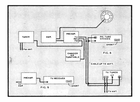
Fig. 8. Diagram of a remote-control system including TV, FM-AM, and phonograph. The preamp can be connected directly to the picture-tube chassis (dotted line) or to the cathode follower pin jack on the remote-control unit. Left, below: Using the TV chassis with tuning controls on the front, as in Fig. 3, the audio output jack is connected directly to the TV input of the preamplifier
