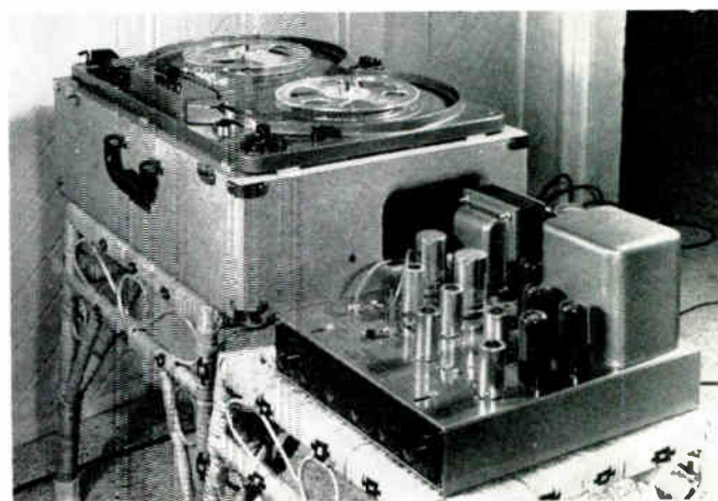
Fig. 1. Part of the time, this 25-watt, two-channel Neucomb amplifier was used with the Berlant Concertone binaural machine for the playback
