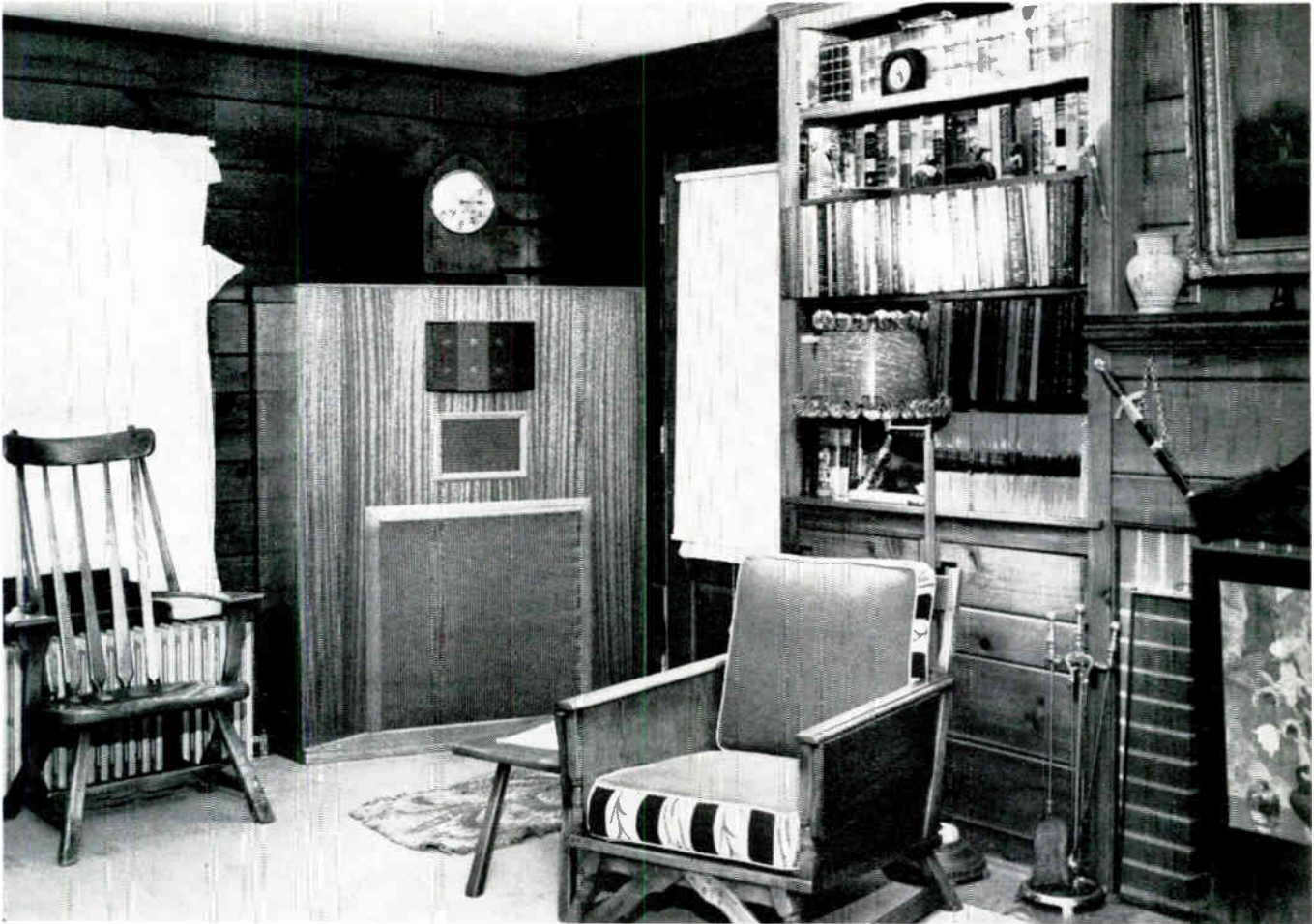
Fig. 1. This speaker system, one of two in the installation, contains 4 woofers, an intermediate speaker, and 8 tweeters
