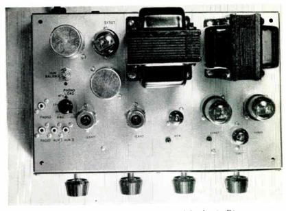
Fig. 2. Top view of the combination preamp and amplifier chassis. Dimensions are 12 ins. wide, 6¾ high, and 8¾ deep behind the front panel
