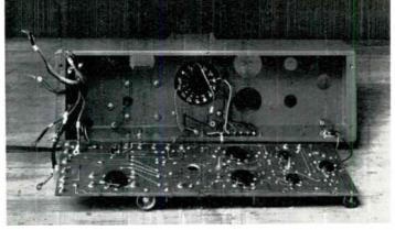
Fig. 2. Top of the mounting plate, with the tubes removed. Part of the printed-circuit wiring is carried on this side
