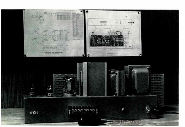
Fig. 1. The UTC Linear Standard amplifier kit was chosen as the first in this series of projects because it requires only the use of a screwdriver. Rated at 20 watts, it can he fed from any tuner, tape recorder, or crystal phonograph pickup, or from the preamplifier used with a magnetic pickup. A novice who has never tackled a joh like this before can complete this amplifier, without burrying, in less than one hour's time
