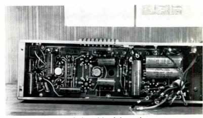
Fig. 4. Appearance of the chassis before the lugs on the numbered wires have been connected to the respective terminals
