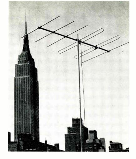
Left: The Tuco Yagi comes all assembled and folded up like this. Above: Here it is with the elements swung out and secured in place by tightening the wing nuts.
