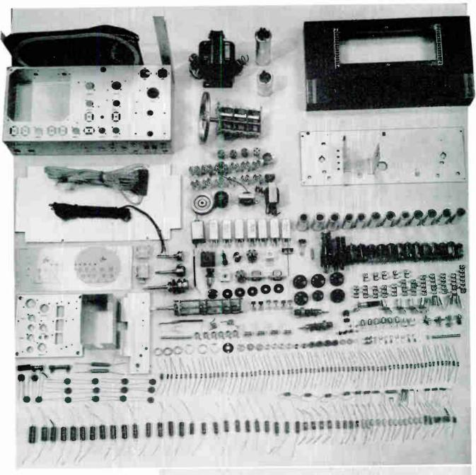
These two illustrations show all the components and parts for a Fisher FM-AM tuner and preamp above, and for a 25-watt power amplifier below. One tube is missing in the upper picture. Reproduced to the same scale as the picture on the opposite page, this explains graphically the difference in price between a conventional AC-DC radio and a hi-fi FM-AM tuner and preamp, with a high-quality power amplifier
