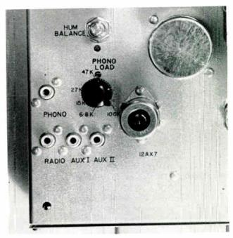
Fig. 3, above: Closeup of the input connections and the chasses adjustments. Fig. 4, below: Rear view showing speaker terminals and outlet
