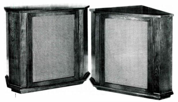
While these cabinets are of moderate size, each contains a 20-in. Styrocone speaker, and four tweeters. The latter are used to provide wide dispersal of treble tones. The cabinet at the left is intended to be placed directly against the wall; the one on the right fits into any corner. Both are built of solid mahogany, heavily braced to prevent vibration in any part of the case
