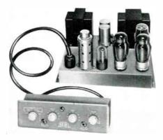
Fairchild, G. E., Pickering, and Sono-Tone. Connections are also provided for a tape recorder and tuner. The 10-watt amplifier, using KT-61 beam power tetrodes in pushpull is described as having .1% distortion at 1,000 cycles with 8 watts output. Dimensions of the amplifier: 11 ins. wide, 9 ins. deep,  $6\frac{1}{2}$  ins. high. The preamp:  $9\frac{3}{8}$  ins. wide,  $2\frac{3}{4}$  ins. high,  $3\frac{3}{4}$  ins. deep. British Industries Corp., 164 Duane St., New York 13.
