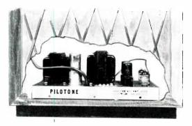
Fig. 4. The bottom of the speaker cabinet provides well-ventilated space for the amplifier, where it can be hidden readily
