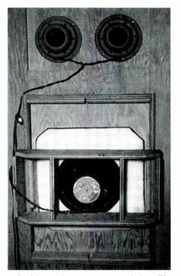
Fig. 4. Front view of the first experimental model, with the Styrocone speaker below, and two tweeters mounted above. This assembly was carried on a heavy piece of plywood, set in place of a closet door. This is a simple, ideal arrangement — where such a door is available. Fig. 5. Rear view, showing the support for the experimental speaker. Note that the cone is not supported at the edges
