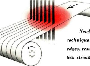
IN THE manufacture of Audiotape, particular care has always been given to the slitting operation, in which the processed tape is cut into reel-size widths. Precision straightline slitting has been one of the reasons why Audiotape tracks and winds perfectly flat and has no fuzzy edges to impair frequency response.
