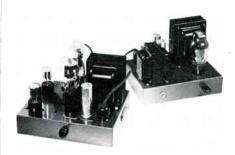
any dealer or mail order house. Construction is simple enough to be completed successfully by anyone who can handle a soldering iron. Instructions are also available for changing the regular Stancor Williamson-type amplifier to the new ultralinear circuit. Performance of the new design is rated less than 1% total harmonic distortion at 1,000 cycles with 25 watt output. Chicago Standard Transformer Corp., Addison  $\Im$  Elston Sts., Chicago 18.
