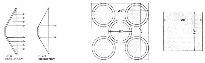
Fig. 1. Low-frequency tones are produced by the movement of the entire cone. Fig. 2. At high frequencies, only a part of the cone moves. Fig. 3. A cone 20 ins. square is equal to the cone area of five 12-in. speakers, occupying twice the mounting area
