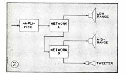
Coupler for the bass, a crossover of 175 cycles is generally used, or 350 cycles if the bass speaker is in a conventional cabinet.
