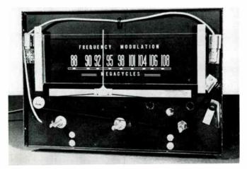
Fig. 2. The front plate can be removed for mounting the chassis in a cabinet. Then it can be put in place again, as in Fig. 1
