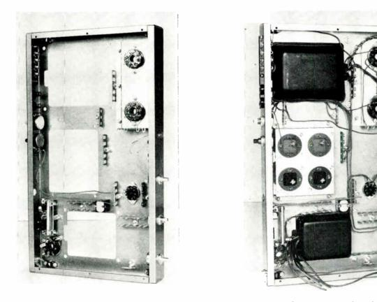
Fig. 1. These parts are mounted before the wiring starts. Fig. 2. With the transformers and filter condensers in place, this much wiring is done
