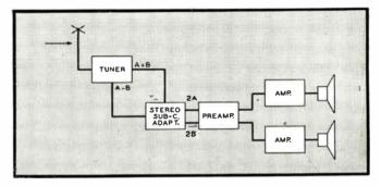
Fig. 6. The A + B channel and the sub-carrier channel modulated by A - B are demodulated. Then, in separate circuits, they are added to produce audio channel 2A, and subtracted to produce channel 2B
