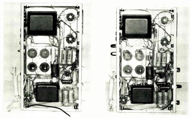
Fig. 3. Capacitors and resistors are added as the work proceeds. Fig. 4. The finished amplifier, ready for the bottom plate, tubes, and cover
