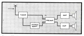
Fig. 4. The demodulated output of the tuner is comprised of an audio channel and a 50-kc. channel which must then be demodulated separately
