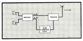
Fig. 5. The transmitter is modulated directly by both audio channels A and B, and also by a sub-carrier generator that is modulated by audio frequencies which are the difference between the two audio channels
