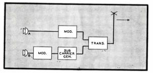
Fig. 3. This 91.5-mc. transmitter is modulated at audio frequencies (A) and also by an audio modulated (B) 50-kc. sub-carrier generator
