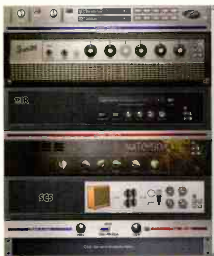
This shows a split patch, with the convolution-based speaker emulator and the Speaker Construction Set.
