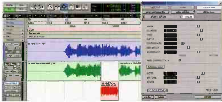
Ex. 6. A vocal track has been copied twice, once to create a major third harmony, and again for a minor third harmony. The DigiRack Pitch Shift window shows the settings for transposing an audio file up by four semitones (major third).
