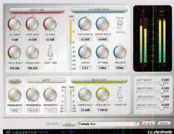
Fig. 3. TC's VoiceStrip, designed for the PowerCore platform, provides traditional vocal strip functions.
