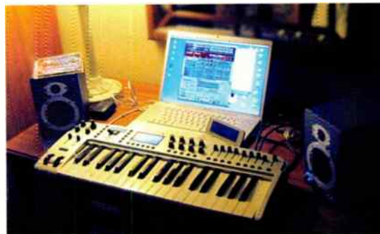
Fig 1: A mobile recording studio can be as simple as an audio/MIDI interface keyboard and your computer. A cell phone with Bluetooth and MP3 player helps to transfer files.
