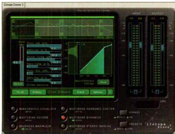
Fig. 3. The Multiband Dynamics Processor in iZotope's Ozone has been set up to add some mild compression in the low end; this smooths out the bass response a bit, which helps make the mastered recording more "transportable."
