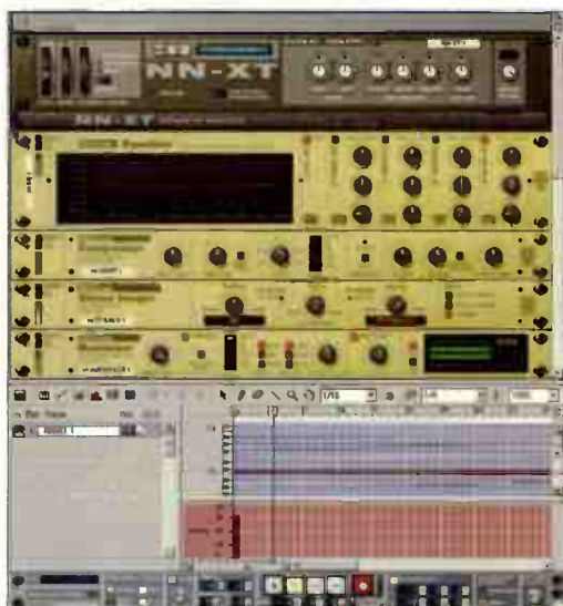
Fig. 9: This mastering setup in Reason combines an NN-XT to playback the file, and a suite of Reason's MClass mastering processors. Note the one-note sequence that plays back the file.
