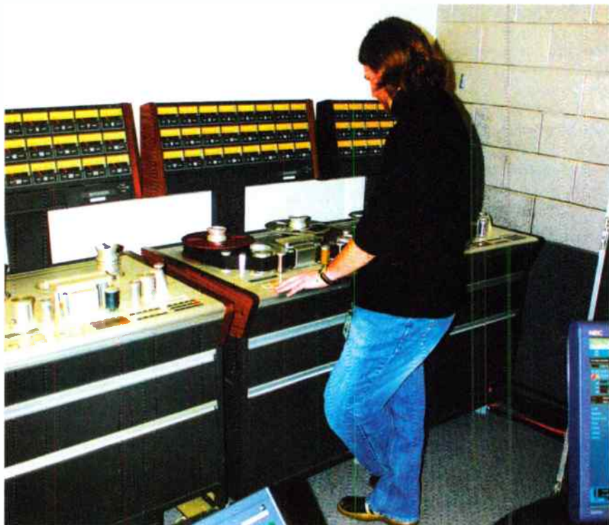
A spare for the spare. Technician Heath Condiotte transfers material from one of Xepa's three Studer A827 machines.
