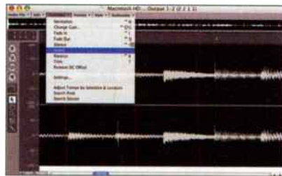
Fig. 4: Logic is one example of a program that allows destructive polarity inversion.
