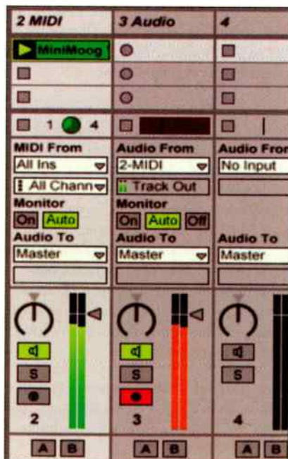
Fig. 1: In Ableton Live 4, the MIDI track (2) is playing back a loop on the Arturia MiniMoog V. The Audio track (3) gets its audio from the MIDI track's instrument, and records this to a hard disk track.
