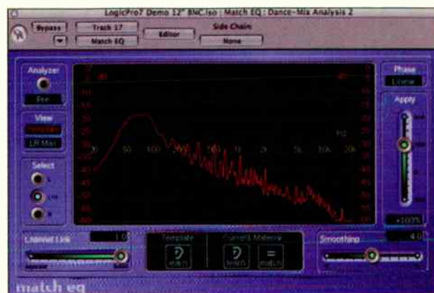
YOU CAN NEVER HAVE ENOUGH EQ — MATCH EQ, SHOWN HERE, LETS YOU "STEAL" A SONG'S EQ CURVE AND APPLY IT TO YOUR OWN MIXES. EVIL? PERHAPS. BUT TRY IT AND YOU'LL BE HOOKED.
