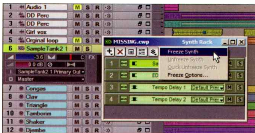
Fig. 2: Like many hosts, Sonar 4 has a "one-click" freeze function. In this example, SampleTank 2 (which is playing a bunch of percussion parts) is about to be frozen from the Synth Rack view. You can also freeze from a pop-up menu when you right-click on a track.
