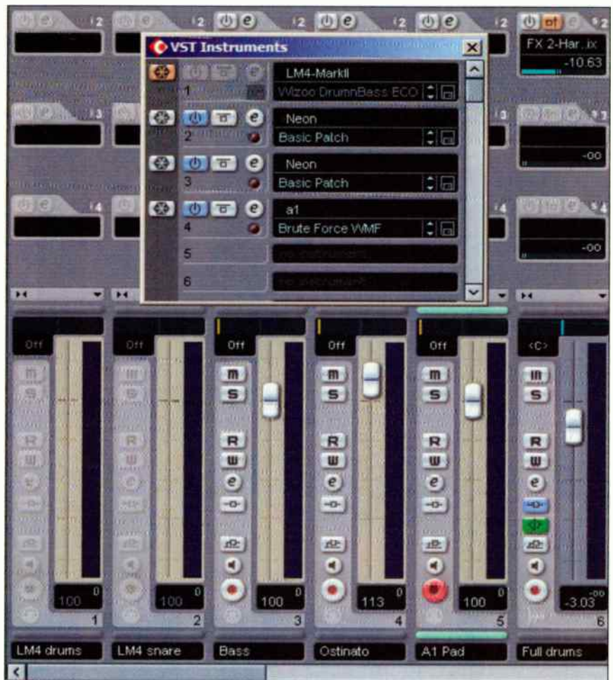
Fig. 3: Cubase has a freeze function that, when applied, causes frozen tracks to be grayed out.
