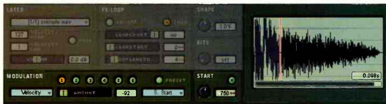
Fig. 1: The highlighted section of the virtual front panel for Native Instrument's Battery drum plug-in shows the controls for modulating, setting, and monitoring the sample start point. (Note: I've modified the front panel graphic to focus attention on the sample start point elements.) On the waveform display, the red line indicates the initial sample start point, as set by the Start control. In the Modulation section, velocity is modulating Sample Start by -92, so higher velocities cause more of the attack transient to be heard.
