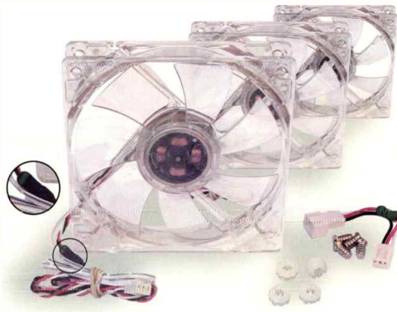
120mm fans move more air with less noise compared to smaller fans. Note the heat sensor (circled) that can be placed in a heat pocket, the silicon mounting grommets to reduce vibration, and a speed-reducing resistor.
