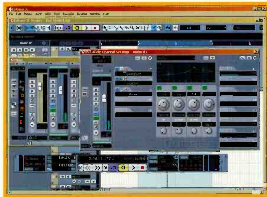
CUBASE SL, A DIGITAL AUDIO+MIDI SEQUENCER, IS BUNDLED WITH SYSTEM|4. WHILE THE FEATURE SET ISN'T QUITE AS COMPLETE AS CUBASE SX, SL OFFERS MOST OF THE SAME FEATURES AND INCLUDES SEVERAL PLUG-INS. NOTE THE 4-BAND EQ AVAILABLE FOR EACH CHANNEL.
