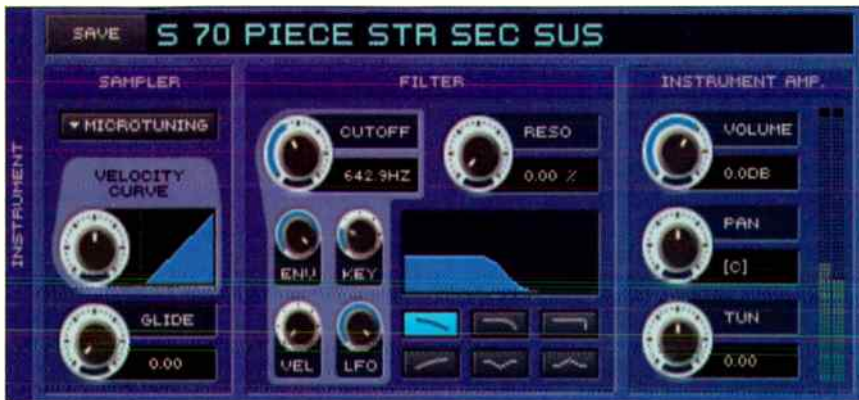
EACH INSTRUMENT IN THE MULTI CAN HAVE ITS OWN TUNING AND FILTER/EQ, AS WELL AS PAN AND VOLUME SETTINGS.
