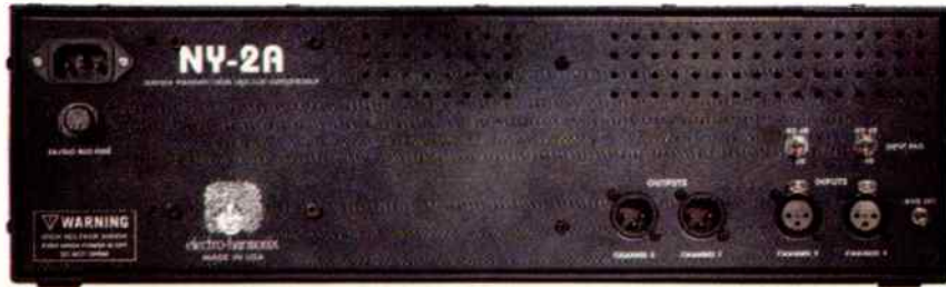
IT DOESN'T GET MUCH SIMPLER THAN THIS: XLR INPUTS AND OUTPUTS FOR EACH CHANNEL. THERE'S ALSO A 20dB PAD SWITCH FOR EACH INPUT CHANNEL AND A GROUND LIFT.
