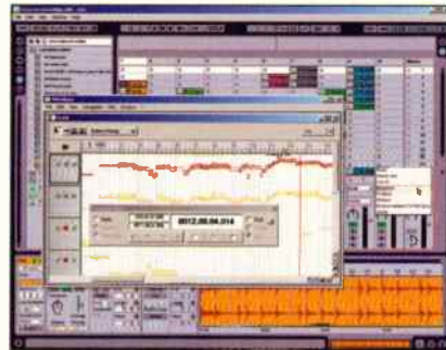
WHEN USED WITH A REWIRE HOST, MELODYNE CAN "PIPE IN" AUDIO TO THE HOST'S MIXER. IT ALSO WORKS AS A REWIRE CLIENT.
