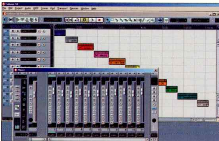
Fig. 1. Files have been dragged into a multitrack host for eventual rendering into a single file, then burned. Each mixer track has levels set individually to even out volume variations.
