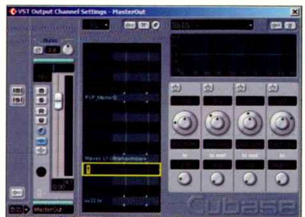
Fig. 2. A Cubase SX 2 output bus. This routing view shows that the uv22hr dithering algorithm is post-fader (the fader position in the signal chain is outlined in yellow for clarity), while the PSP MasterQ and Waves L1 are pre-fader.
