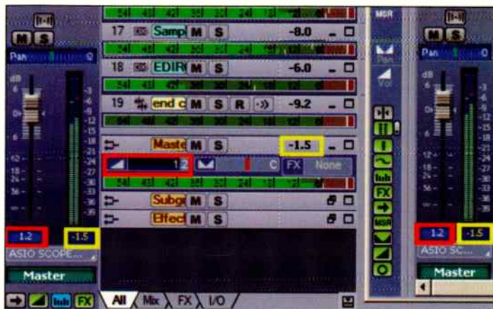
Fig. 3. From left to right, Sonar's Inspector, Track View, and Console faders all show the fader value (outlined in red for clarity) and the "margin," or highest level attained (outlined in yellow).
