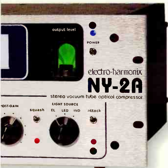
THE NY-2A HAS THREE DIFFERENT TYPES OF OPTO-COUPLER LIGHT SOURCES BUILT IN. EACH HAS UNIQUE COMPRESSION CHARACTERISTICS, MAKING THE UNIT MUCH MORE VERSATILE THAN YOU'D EXPECT AT FIRST GLANCE.
