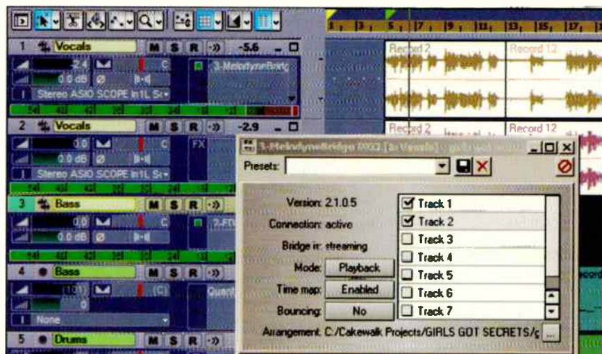
MELODYNE WORKS AS A "PSEUDO PLUG-IN" WITH HOST PROGRAMS THROUGH MELODYNEBRIDGE, WHICH TRANSFERS TRACKS INTO MELODYNE. THESE CAN BE EDITED AND PLAYED BACK IN CONJUNCTION WITH THE HOST.
