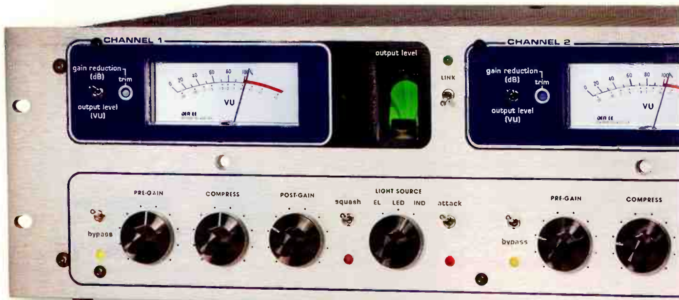
THE ELECTRO-HARMONIX NY-2A USES A TUBE-BASED OPTICAL DESIGN FOR COMPRESSION. THE UNIT IS SIMPLE TO USE: PLUG IT IN, HOOK IT UP, AND DIAL UP THE PRE-GAIN AND COMPRESS KNOBS TO ADD GAIN REDUCTION. THE POST-GAIN CONTROL ADDS MAKE-UP GAIN.
