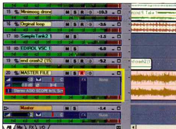
Fig. 4. In this example, Sonar's master bus feeds a hardware out, which returns back to track 20 (outlined in yellow) via a hardware input (outlined in red) where it is recorded prior to exporting.
