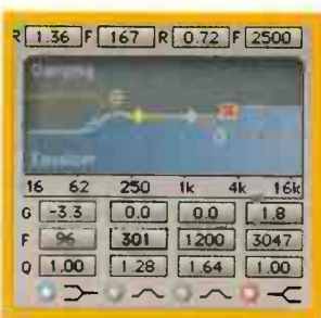
DAMPING AND EQ CHANGES CAN BE MADE FROM THE SAME WINDOW BY DRAGGING THE CONTROL POINTS.
