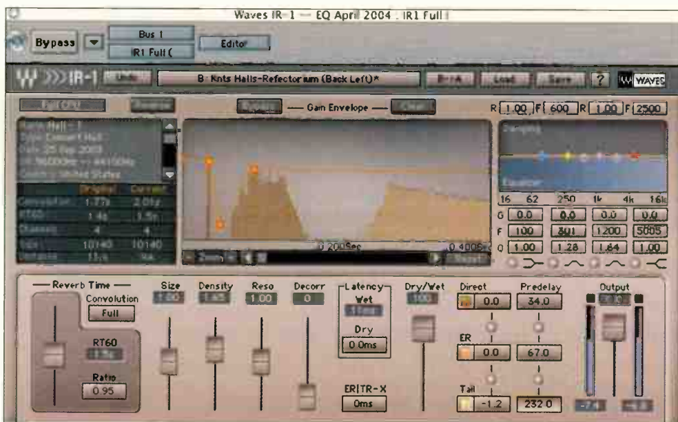
IMPULSE RESPONSES ARE REPRESENTED GRAPHICALLY IN THE CENTER WINDOW. HERE I'VE CHANGED PREDELAY FOR THE EARLY REFLECTIONS AND REVERB TAIL TO SHOW HOW AN IMPULSE CAN BE SEPARATED INTO THREE PARTS.
