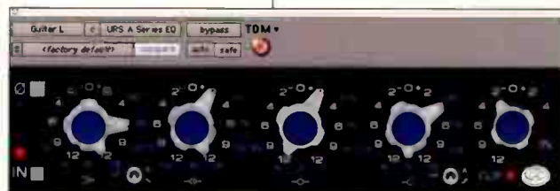
THE URS A SERIES EQ PLUG-IN MODELS THE RESPONSE OF AN API 550B EQ MODULE. THERE ARE FOUR SEMI-PARAMETRIC BANDS. THE HIGH AND LOW BANDS CAN BE SWITCHED BETWEEN PEAK AND SHELF RESPONSE.
