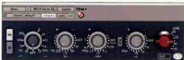
THE NEVE-LIKE URS N SERIES PLUG-IN HAS A PEAKING MIDRANGE SEMI-PARAMETRIC BAND AND SWEEPABLE HIGH AND LOW SHELF BANDS, PLUS HIGHPASS AND LOWPASS FILTERS. YOU CAN SWITCH THE MID BAND TO HI-Q FOR NARROWER BANDWIDTH IF YOU NEED TO GET SURGICAL.
