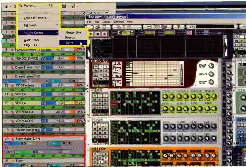
FIGURE 2: Arturia's Storm is ReWired into Cakewalk Sonar to provide additional percussion. Upon inserting the ReWire device (outlined in yellow for clarity), tracks show up in Sonar for audio outs and MIDI ins (outlined in red).
