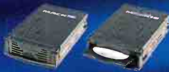
Front bay accepts M-90 pull-out hard disks or a Mackie Media Project ORB™ drive for quick transfer of up to 2.2 gigs of music.
