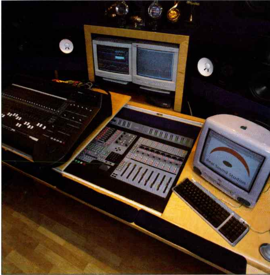
LET IT SLIDE: Kike's Mackie D8B console slides off to the side to reveal the Digidesign Pro Control system.
