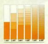
Every bit you add doubles the resolution of a digital recorder. Compared to 16-bit formats, ADAT Type II's non-compressed, linear 20-bit recording offers a wider dynamic range, less quantization distortion at low levels, more headroom and even lower noise. Result: detailed, full-spectrum audio fidelity that far exceeds the quality of any analog recorder.
