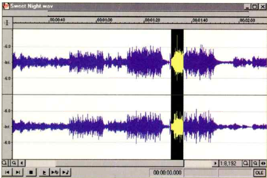
FIGURE 1: Note how a single transient (in the highlighted area) reaches the maximum available dynamic range. As a result, normalization cannot bring up the overall level any further.
