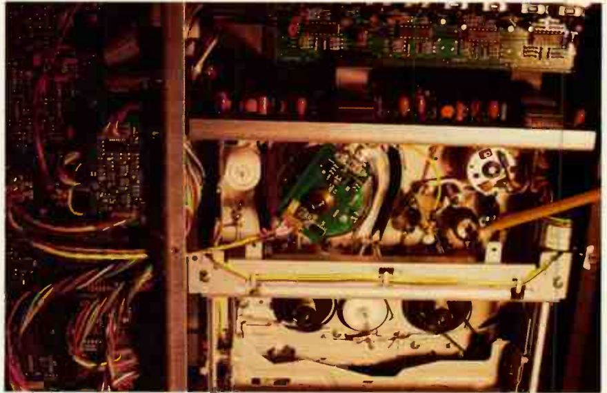
FIGURE 1: ADAT interior with pinch roller identified.
