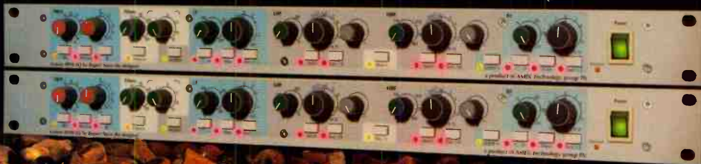
The System 9098 EQ is a Stereo 1U 19" Patch Rack unit and 2 Units are shown here.
