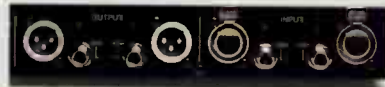
So you'll have no trouble patching things up, the SPX990 takes either XLR or TRS phone jack connectors.
