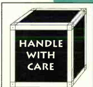
ATA CASE: Handles (2 per side) and catches not shown. Allow 1/4" height and 1/2" width allowance. Be sure to compensate for width of rack rails.
