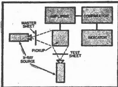
Fig. 2.—Block diagram of a one source-two pickup system.
