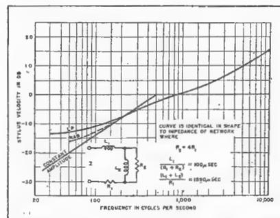
Fig. 2.—This graph shows the relative characteristics of the Long Playing, NAB transcription and Constant Amplitude records.
