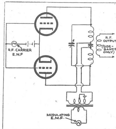
Fig. 6.—Basic arrangement of balanced modulator.
