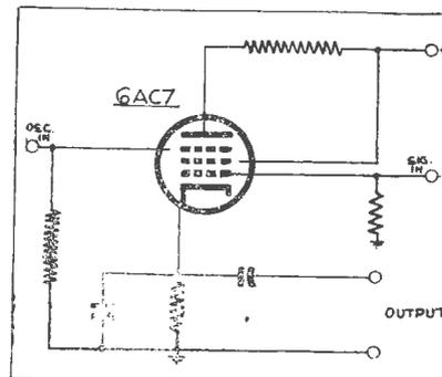
Fig. 5.—By using the suppressor grid as an injector grid, an ordinary pentode may be employed as a mixer/detector.
