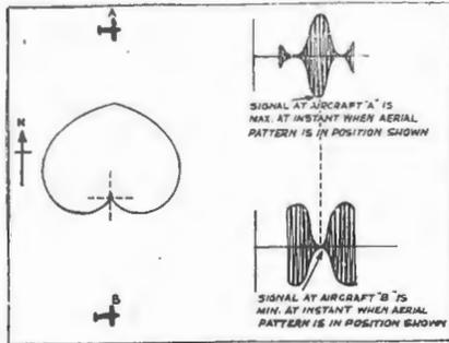
Fig. 3.—This diagram illustrates that the phase of the modulation due to a rotating aerial pattern of cardioid form is dependent on the bearing of the receiver from the aerial.
