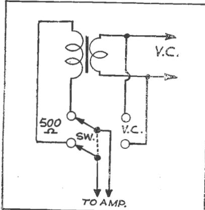
The use of a double pole-double throw switch enables the speaker connections to be changed.
