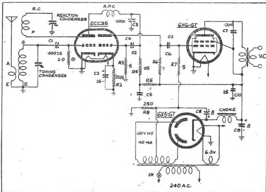
This circuit requires only three valves and should present little difficulty to the constructor. It is capable of excellent results on all local stations.
