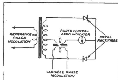
Fig. 9.—Simplified circuit of phase discriminator.
