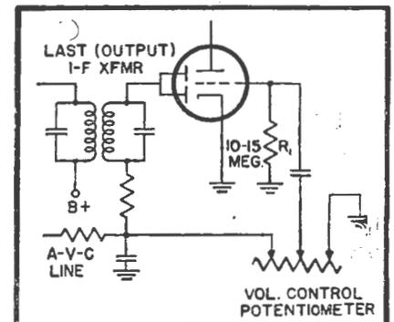
Fig. 6.—An increase in the value of R1 will cause distortion as described in the text.
