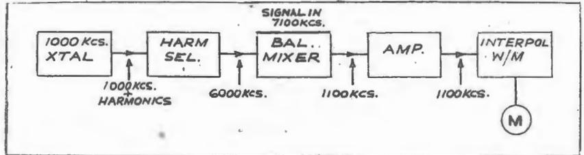
Fig. 3.—Block diagram of one form of Wavemeter.
