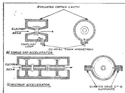
Fig. 9.—Linear Accelerators using resonant cavities for micro-wave operation. In the case of the multi-gap accelerator (b), the adjacent cavities are coupled together by the electric field at the edges of the baffles. The baffles are effectively insulated from the body of the cavity by quarter wave stub support.
