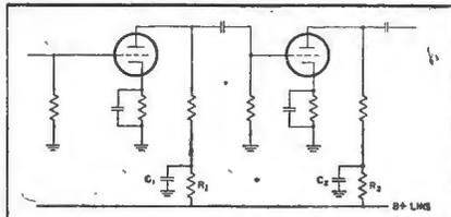
Fig. 7.—The installation of resistors R1 and R2 and condensers C1 and C2 will often remedy "motor-boating".
