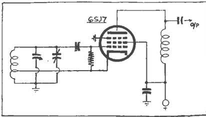
Fig. 4.—The electron-coupled circuit provides good electrical stability.
