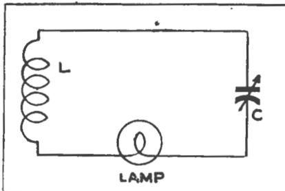
Fig. 1.—The basic circuit for an absorption type wavemeter.
