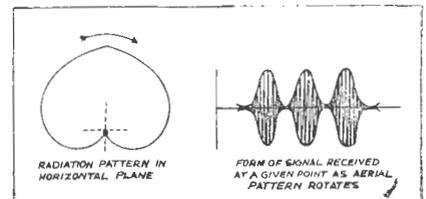
Fig. 2.—Illustrating a horizontal radiation pattern of cardioid form and the nature of the signal received at a given point as the aerial pattern is rotated.
