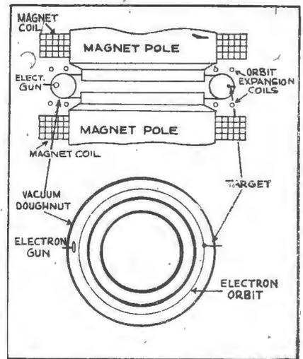
Fig. 13.—The essential components of a Betatron.
