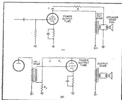
Fig. 1.—The circuits above illustrate two common methods employed to obtain regenerative feedback. In A, resistor R and capacitor C constitute the feedback circuit. In B, resistors R1 and R2 and capacitor C constitute the feedback circuit.
