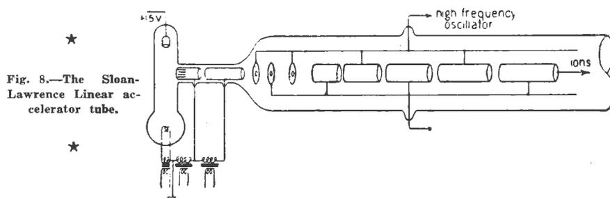
accelerate them when they are crossing the gaps. As the ions speed up the drift tubes must be made longer.
