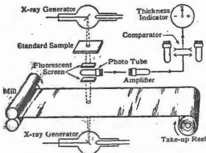
Fig. 1.—The thickness gauge uses two x-ray generators. The radiations from one pass through the sheet in question; those from the other through a standard. The surviving radiations fall, alternatively, on to the x-radiation sensitive screen surrounding a photo-multiplier. The results are amplified, compared, and any difference applied to an indicator.
