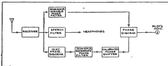
Fig. 10.—Simplified block schematic circuit of airborne equipment.
