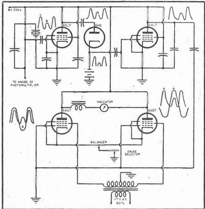
Fig. 3.—The gauge circuit used in the x-ray thickness gauge.
