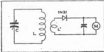
Fig 2.—(b) By replacing the indicator lamp in Fig. 2 (a) with a rectifier and meter combination, a more positive indication is obtained.
