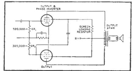
Fig. 5.—Push-pull output stage and phase inverter combined.
