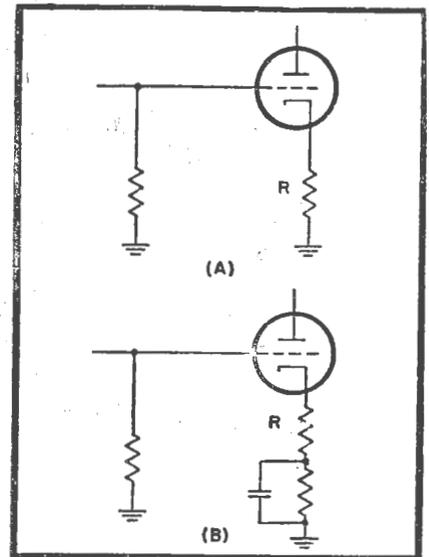
Fig. 2.—Negative feedback voltage may be developed across the cathode resistor of an amplifier by omitting the bypass condenser as shown in (A) or by placing the bypass condenser across only part of the cathode resistor as shown in (B).
