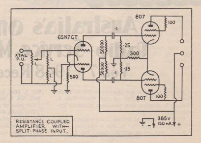
In response to a number of enquiries, here is a typical circuit of the split-phase idea applied to resistance-coupled amplifiers. The above circuit gives splendid results with a suitable type of crystal pick-up.
