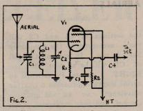
small steps, retuning C2 each time (only a small movement will be necessary) until maximum strength results. The unit is now matched to the input impedance of the receiver.
